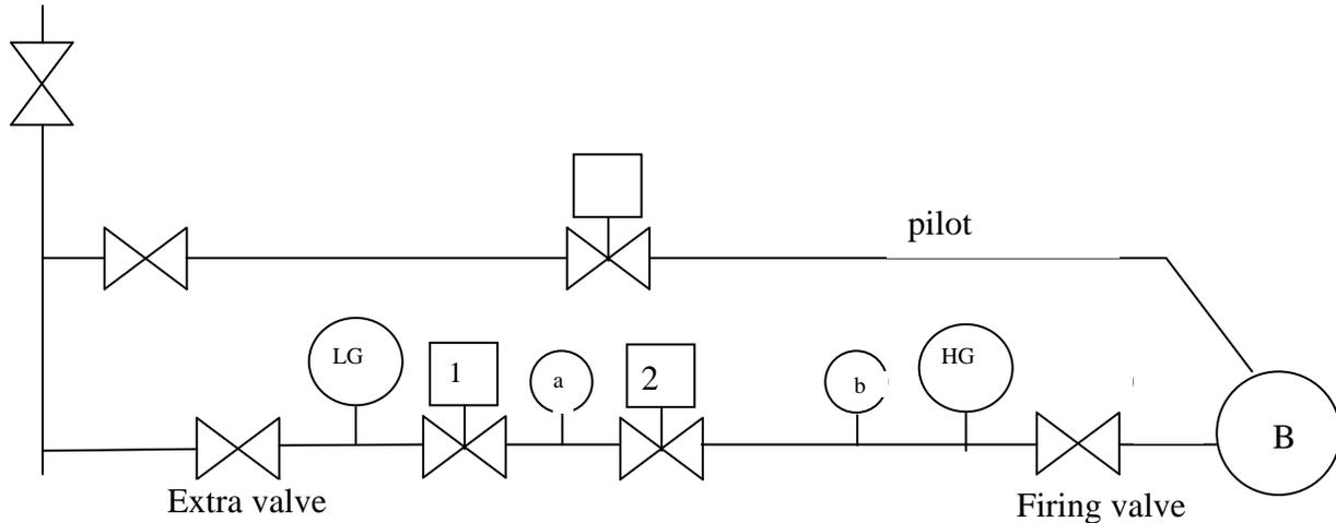
1. TEST THE LEAK TIGHTNESS OF THE FIRING VALVE:
