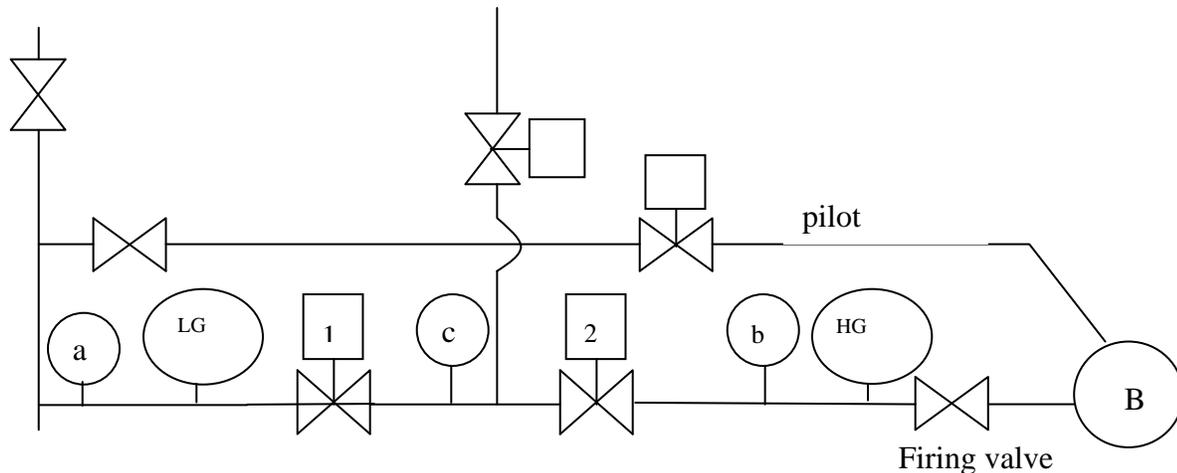
Procedure for testing integrity of safety shut-off valves, guarded status with interrupted pilot and double block & bleed:
