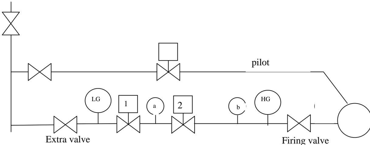
Procedure for testing integrity of safety shut-off valves, guarded status with standing pilot:
