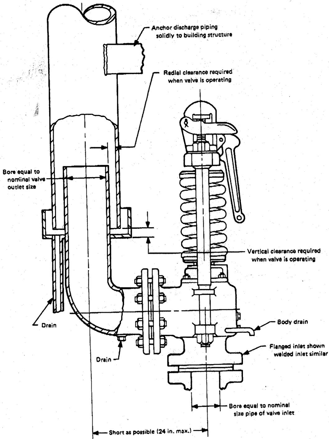
**FIG. C4.1-3 RECOMMENDED SAFETY VALVE INSTALLATION**
