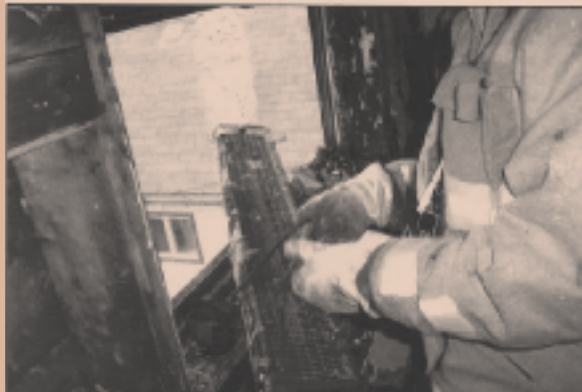
The cause of this fire, the baseboard heater's electrical chord is pinched by the bed frame, causing resistance heating.
